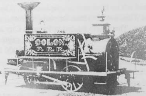
Locomotive "Colon" built by Portland Locomotive Works, August 21, 1865. Note left side controls. (Clifton E. Hull collection)
