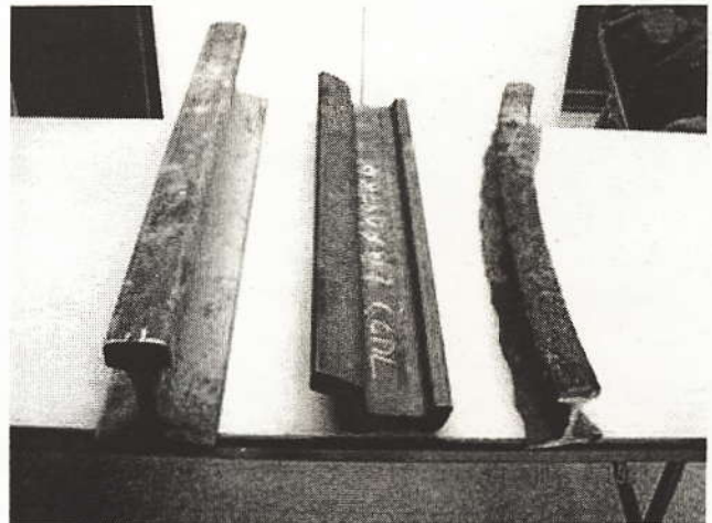
'Pardon Our CAT Tracks' signs are all over. CAT stands for Central Arkansas Transit. At right are pieces of streetcar track John Jones brought to our last club meeting. The one on the left is the current track, middle is a piece used on the curves and on the right is a piece of original track from North Little Rock.
