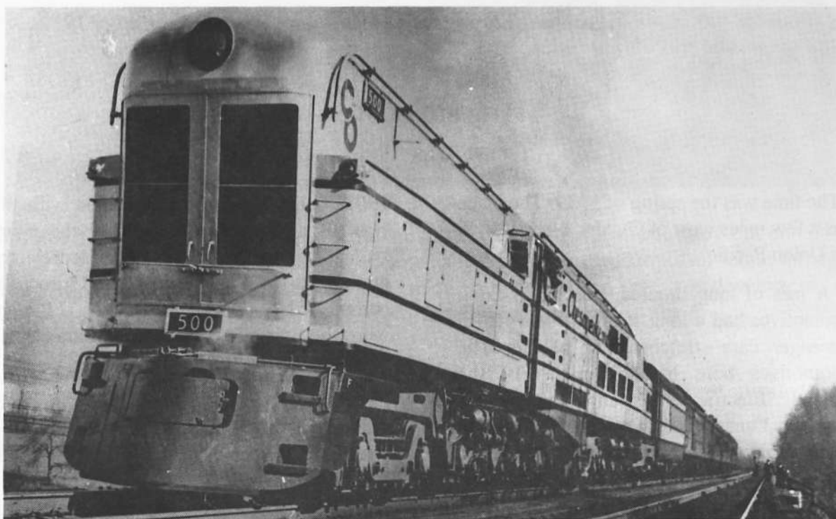
C&O experimental steam-turbine-electric 4-8-0-4-8-4 No. 500; first of three by BLW in 1947. (Gene Hull collection)
