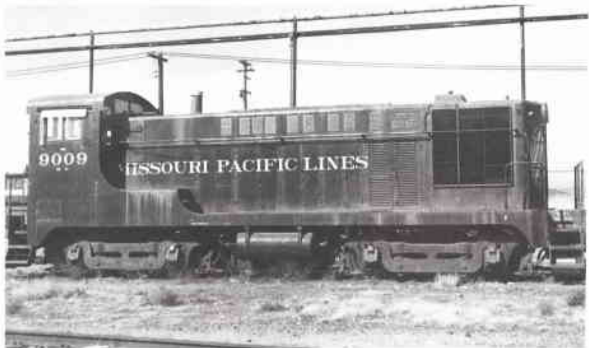
(6) BLW 660 h.p. switcher No. 9009 in North Little Rock, Arkansas in 1945; built in 1940. (Gene Hull photo)
