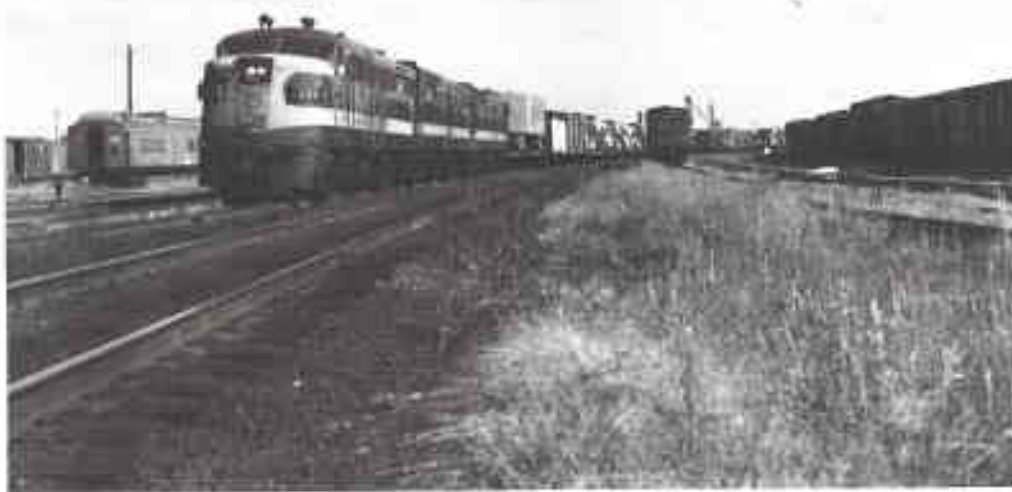
(7 Top) - This EMC E3-A 2000 h.p. diesel was built in 1939 and helped power the MISSOURI RIVER EAGLE, Mo.P.'s first streamlined passenger train. It is shown at the North Little Rock, Arkansas engine house in 1960.
