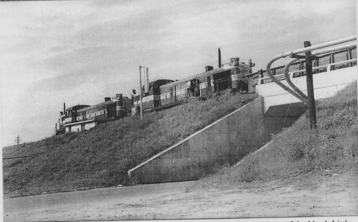
TOP - A Mo. Pac. Gondola No. 61531 rolls down the initial 3 percent slope of the North Little Rock "hump" yard toward a distant classification track in the summer of 1962. BOTTOM - In 1962, a pair of ALCO RS-3's, No. 290 and No. 991, are slowly pushing cars over the "hump" at North Little Rock. ( Gene Hull photo )
