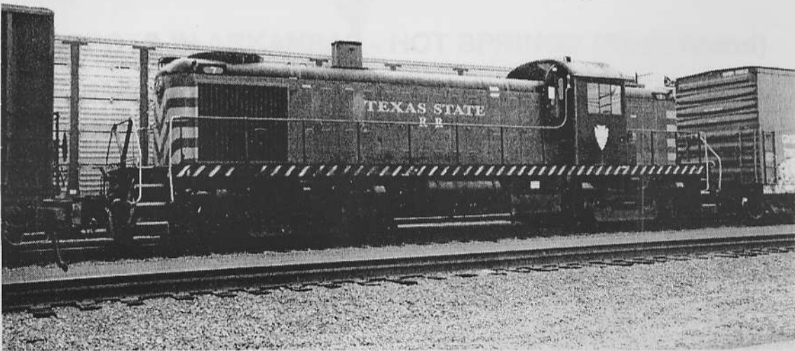
TOP -US Army 4014, RS-4-TC-1A at North Little Rock on April 10, 2003, 500 hp. It was heading to Fort Chaffee, Arkansas. BOTTOM -Texas State RR #7 (TSR #7) in the North Little Rock Union Pacific yard on February 8, 2003. It's an Alco RS-2, 1500 hp, built in 1947. It was heading for Brookville, Pennsylvania. (John C. Jones photos)
