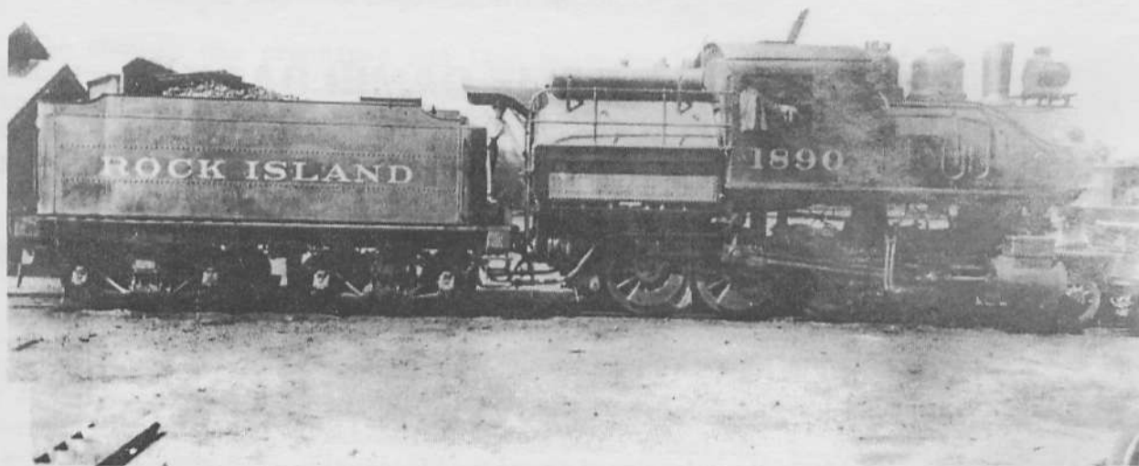
Rock Island Camelback 2-8-0 No. 1890 at Little Rock (?). The fireman is beneath the roof canopy over the gangway. (Gene Hull collection)
