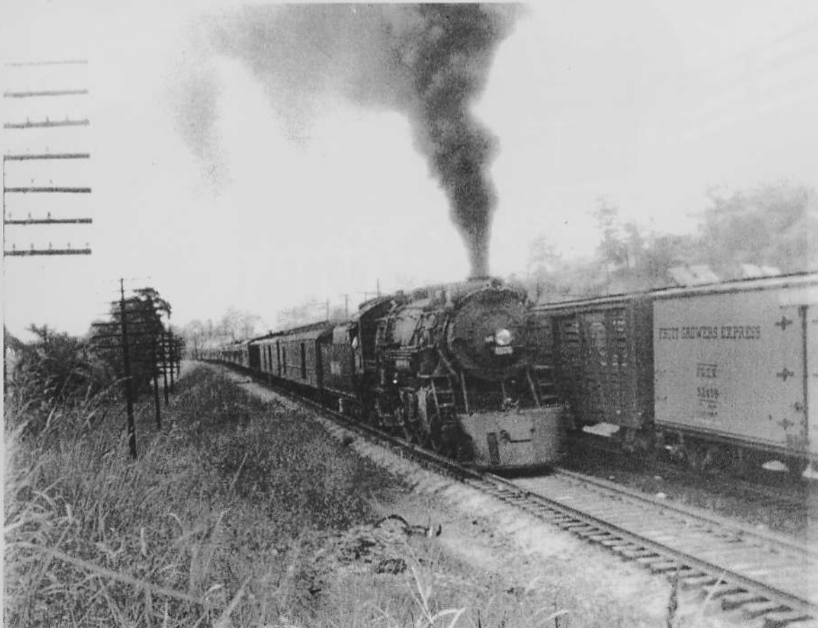
Engine #6606, 4-6-2 Pacific coal burner has a long consist as train #7, The Southerner , tackles the hill in Little Rock in 1945. The east-northbound "Meat" train on the next track will proceed on to North Little Rock where the "reefers" will be iced before this hotshot heads on north toward Dupou, Illinois, after #7 clears the HH tower interlocking. (John A. Mills photo)
