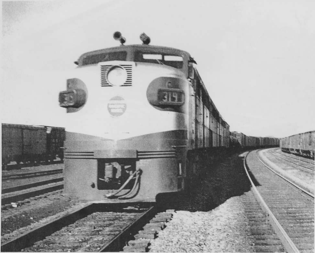
ALCO FA #319 powers this three-unit southbound Red Ball freight through the North Little Rock shop area in 1950. Delivered in April 1948, this is one group of locomotives some folks didn't care for, me included. While working with an outbound inspector at North Little Rock as an apprentice, I never opened a crankcase inspection cover that I did not smell "burnt" oil and see metal shavings. The General Electric electrical components were OK, but the Alco power plants left much to be desired. (John A. Mills photo)
