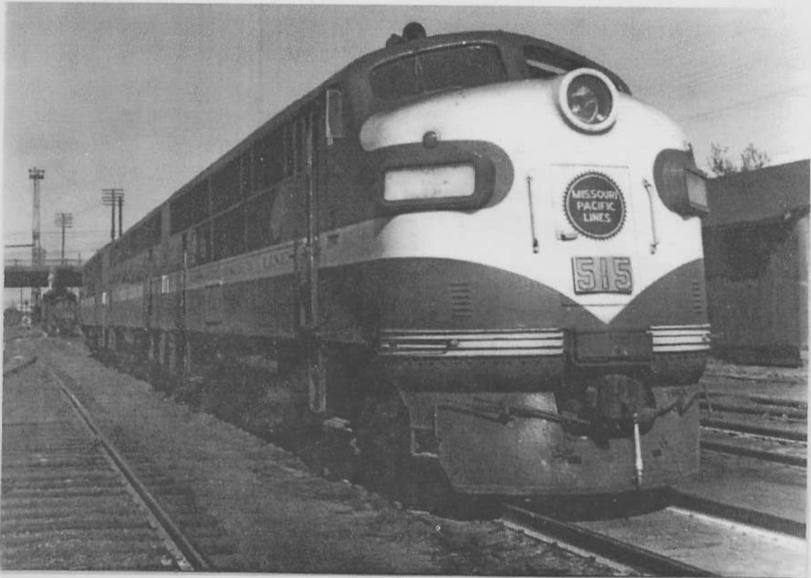
Missouri Pacific, total horsepower 4500, GM-EMD A-B-A No. 515 sitting beside livestock pens at North Little Rock, Arkansas in 1948. (Gene Hull photo)
