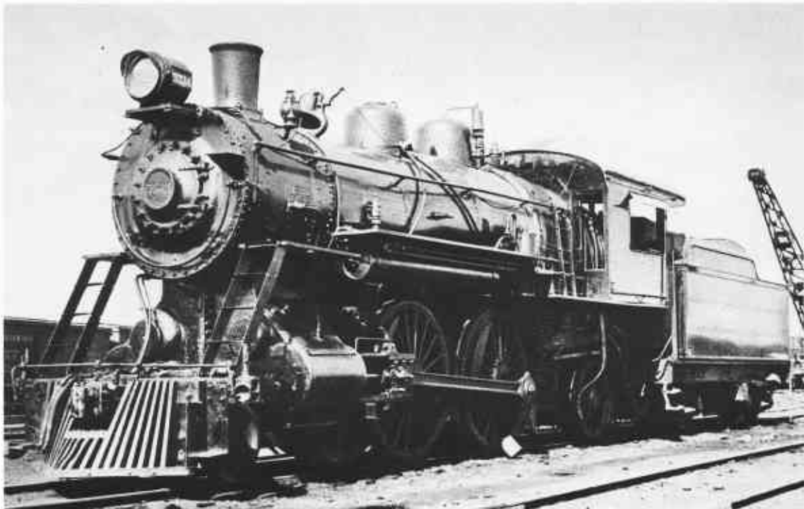
Missouri Pacific No. 5534 , a 4-4-2 Atlantic type. One of 40 built for MoPac-Iron Mountain from April 1904 to April 1907 by Alco-Brooks Works. Strictly fast passenger power, the 5534 was in the last class built and here rests at Van Buren, Arkansas August 1953. The 5534 was later modernized (not when this picture was taken) to include boosters on trailing trucks. Up to and during World War II they were used everywhere but were all gone by 1946. (Mike Adams collection)
