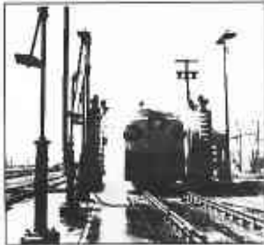
ALCO-GE FA-1 No. 313 is getting a refreshing bath at the engine washer at the North Little Rock engine house in 1955. This was one of the earliest ALCO F1 units acquired in 1948. Appearance was important to the reorganizing Mo. Pac. (Gene Hull photo)
