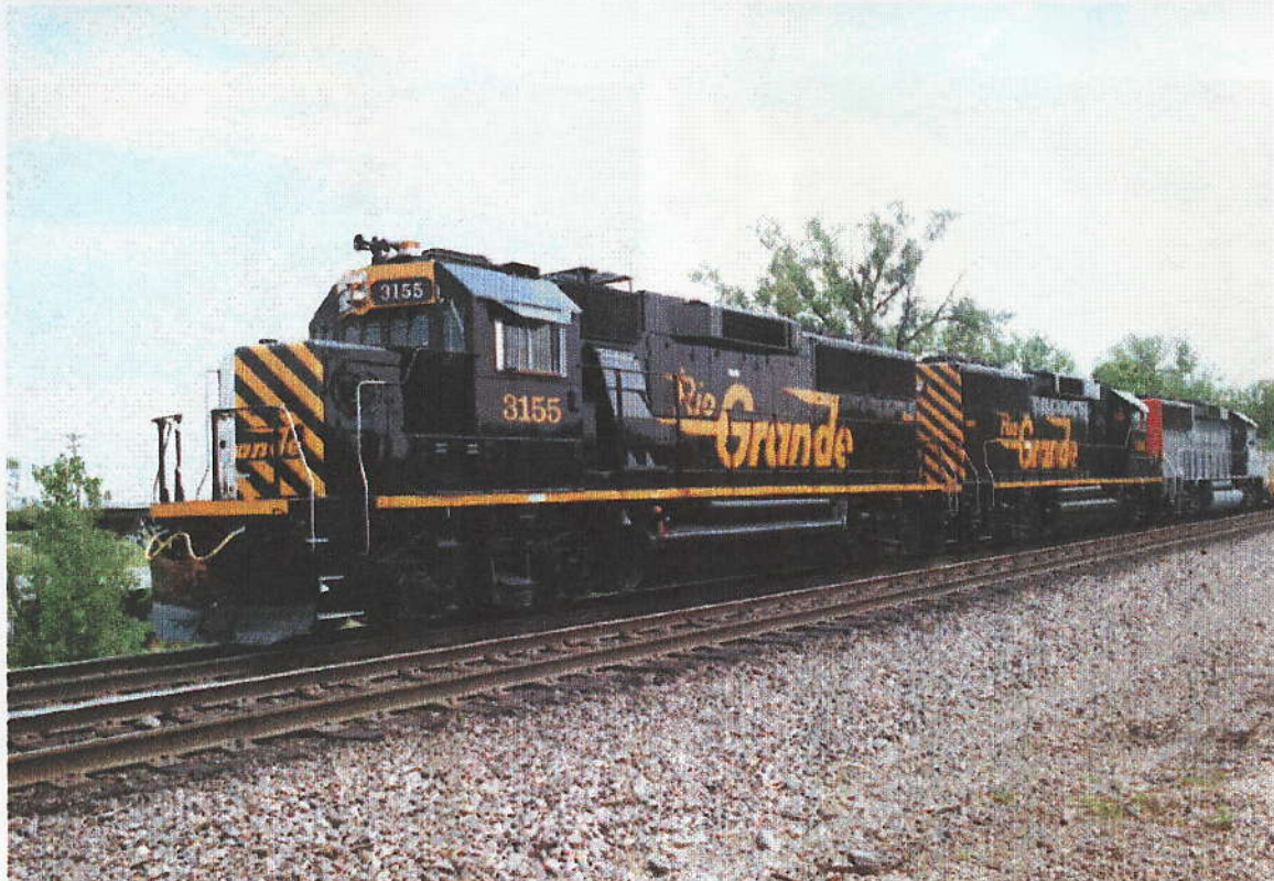
June 11, 1990 - Two new General Motors Electro-Motive Division-built GP-60 locomotives, the first painted in the colors of the Denver & Rio Grande Western Railroad since the October 1988 combination of Rio Grande, Southern Pacific and SP Subsidiary St. Louis Southwestern (Cotton Belt) under the ownership of Rio Grande Industries and operation under the banner of the Southern Pacific system, leave Kansas City, Kansas headed for SP's Los Angeles/Long Beach ICTF rail yard in southern California. The 3,850 hp, 16-cylinder, four-axle units, part of a delivery of three such locomotives, are micro processor-equipped for greater fuel economy and performance. Trailing the two Rio Grand units is one of the 50 GP-60's painted and lettered for Cotton Belt and received in May, 1990. The DRGW GP-60s are also the first of their class on Rio Grande's locomotive roster, and were constructed at EMD's London, Ontario assembly plant and delivered to Southern Pacific at Chicago. SP has now ordered 213 new diesel locomotives since the spring of 1987. (This was an official Southern Pacific press release, June 11, 1990 written by then-Public Relations head Jim Johnson)
