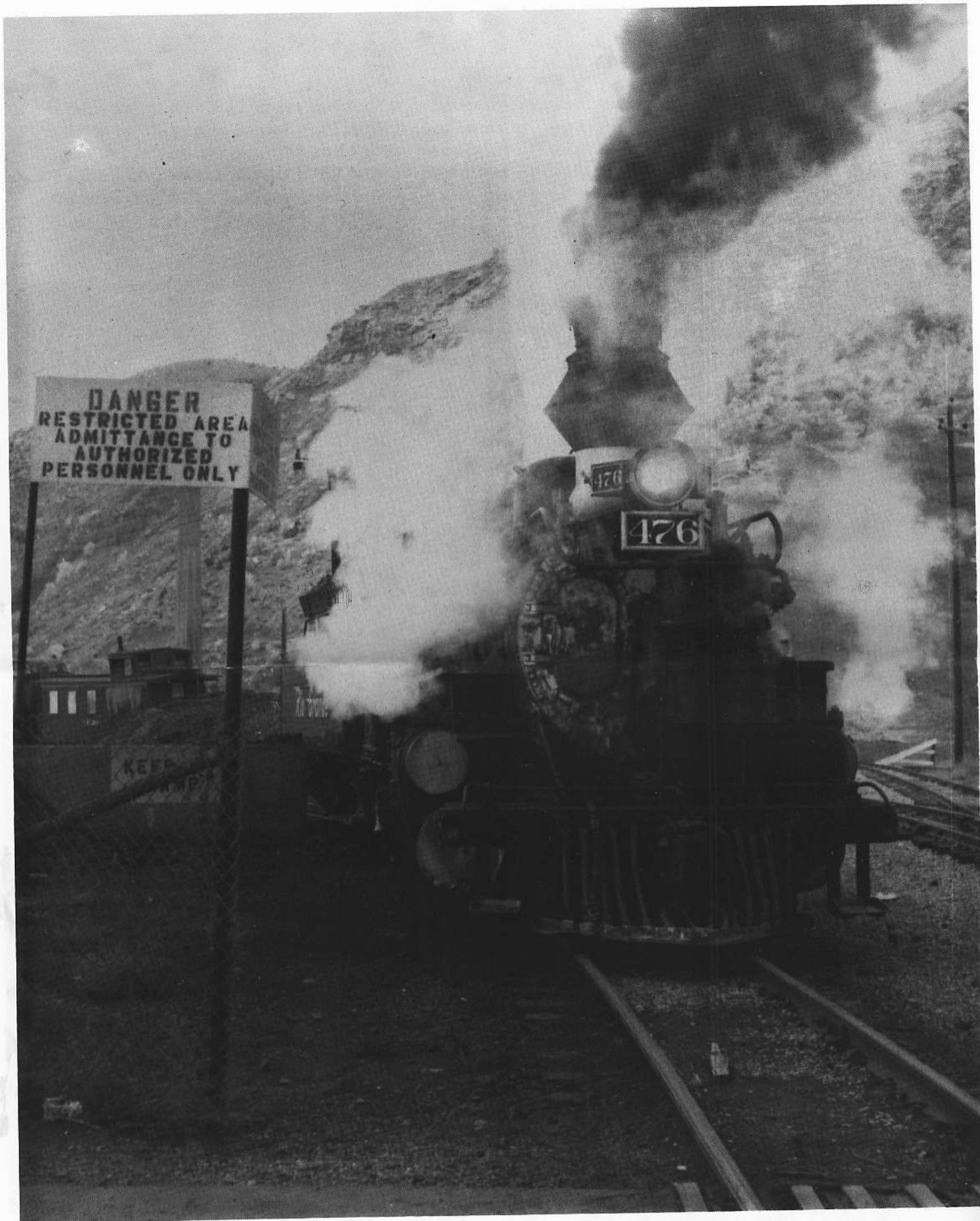
Denver & Rio Grande Western narrow gauge 2-8-2 No. 476 serviced at Durango, Colorado and ready for the train to Silverton, September 1993. (Gene Hull photo)
