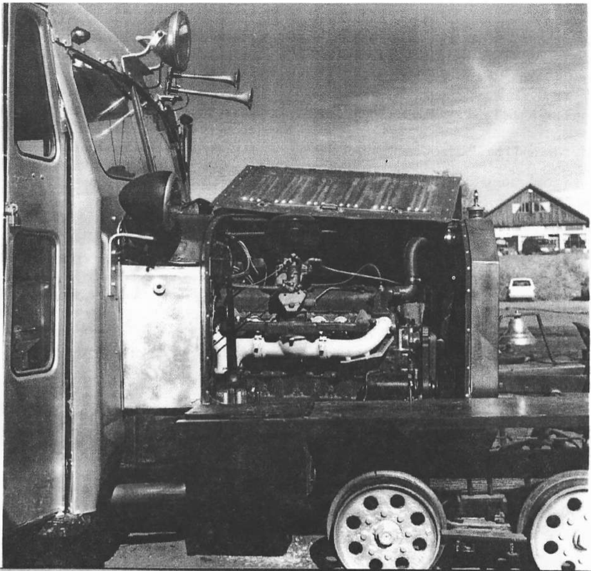
The GMC six cylinder gasoline engine in the Goose was rebuilt at Cortez, Colorado, about 10 miles south of Dolores. ( Gene Hull photo )
