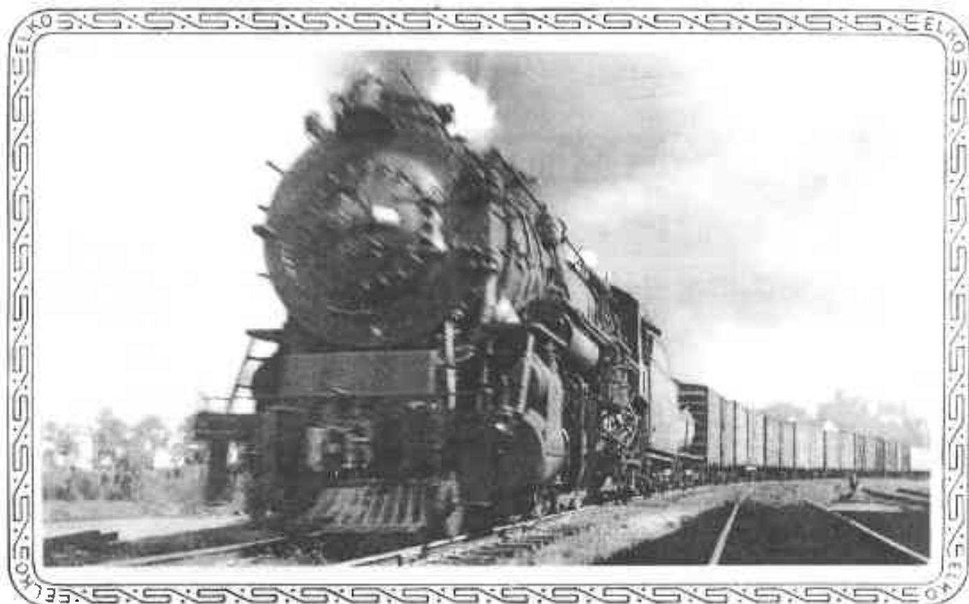
A "fat-boilered" Mike engine going by Little Rock Union Station on the freight main in October 1941. It was going about 40 mph and had engine 1489, a 2-8-2. (Mike Adams photo)
