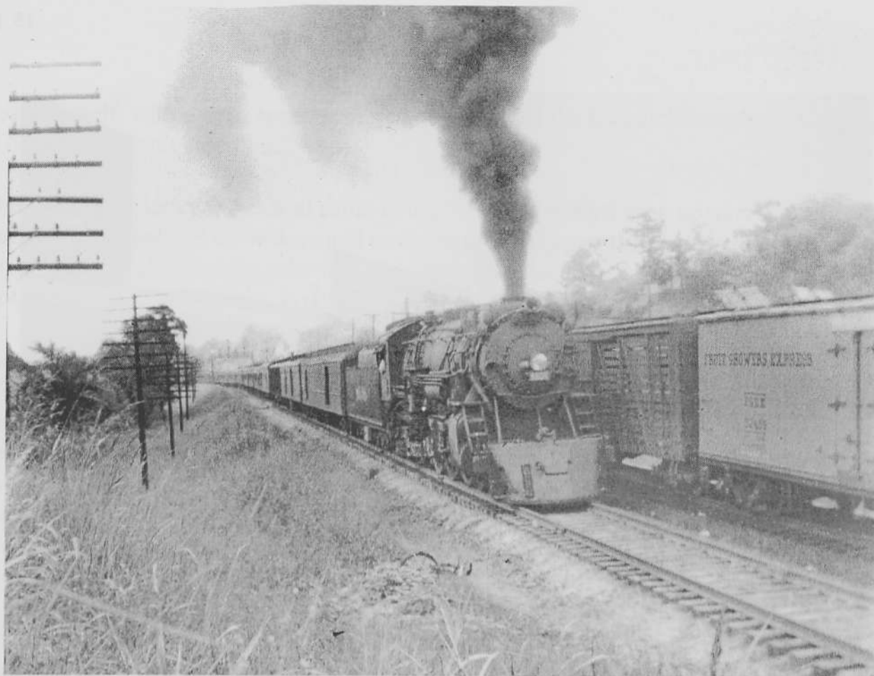
Engine #6606, 4-6-2 Pacific coal burner has a long consist as train #7, The Southerner , tackles the hill in Little Rock in 1945. The east-northbound "Meat" train on the next track will proceed on to North Little Rock where the "reefers" will be iced before this hotshot heads on north toward Dupu, Illinois, after #7 clears the HH tower interlocking. (John A. Mills photo)
